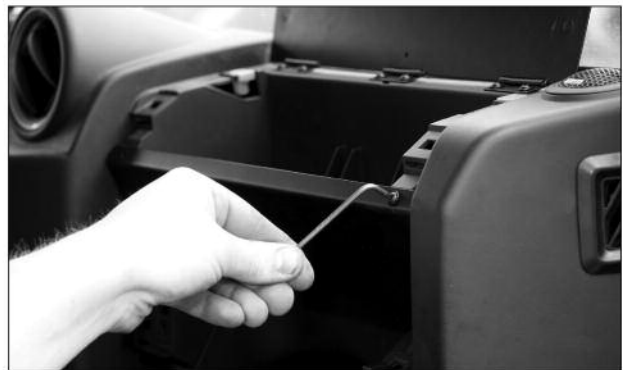
6. Mount front panel (5 screws)
