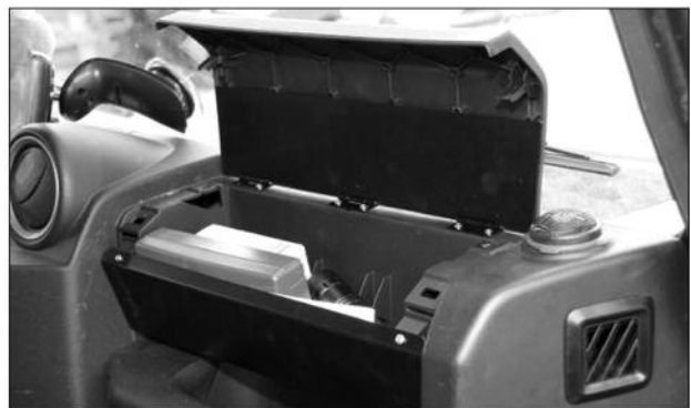
6. Mount front panel (5 screws)
