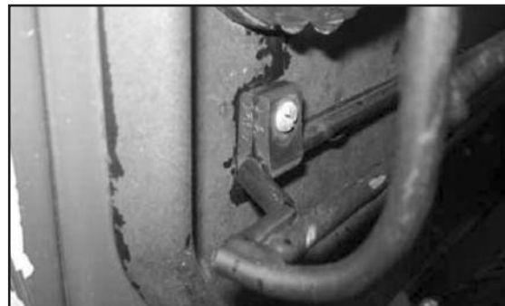
For the 2 larger rectangular light guards use 2 of fixing B as shown in Pic 3 and 2 of fixing A as shown in Pic 4.
