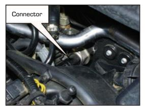
Place the connector from the PSI-Box over the sensor. Connect the male connector from the Box on the female connector from the wiring loom.
