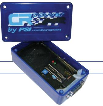
The Box is placed between the pressure sensor from the rail and the wiring loom from the engine.
