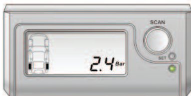
(e) The system will enter into the reference pressure setting of back tyres automatically after setting front tyres pressure and show the current reference pressure. Set the new reference pressure step (c) and (d).
