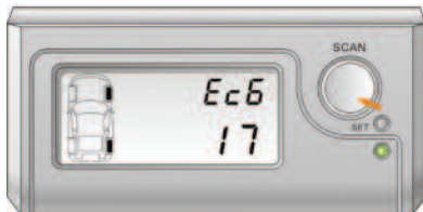
(d) Press SCAN select the back right wheel (indicator of selected tyre will be kept unchanged).
