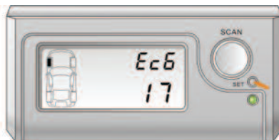
(b) Press SET to enter the Learn New ID mode. It will show position of front wheel and its ID
