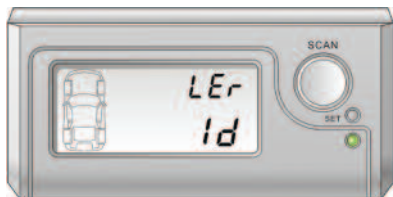
(a) Enter setup mode and select the interface of Learn New ID'.
