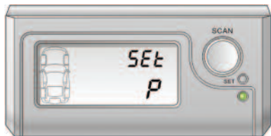
(a) Enter setup mode and select the interface of Set Reference Pressure
