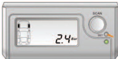
(b) Press SET to enter the interface of the setup mode of Reference Pressure, the system shows the present reference pressure.
