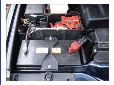
Undo the battery lead to chassis earth retaining nut with a 10mm spanner.
