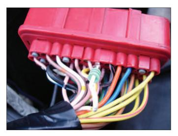
Now put the female type connector from the Turbo Boost Box into this hole. Push it right in and you should hear or feel a click as it locates. Give it a gentle tug, and it should stay put.
