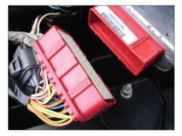
Using a small screwdriver, gently prise off the white plastic cover, to expose the terminals.
