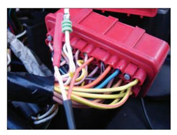
Take the lead from the Turbo Boost Box with the heat shrink tubing, and push the White/Yellow cable you took out of the red plug, in to mate up with the male connector inside.
