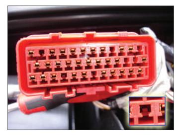
Now we need to identify the pin which needs to be removed. We are looking for pin 6, which is located on the bottom row of the plug. As our plug is upside down, it is therefore at the top. Counting from right to left, starting at 1, count the pin numbers (including pins not in use) up to 6. This will be a White wire with a Yellow marking. The markings on the wire will vary depending on the year of manufacture of your vehicle. Examples of early and late model wiring is shown below.
