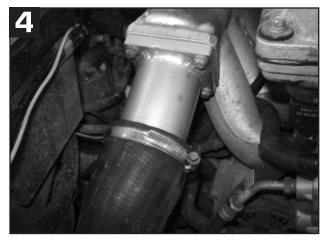
Clean surface of inlet manifold, fit gasket and new inlet adaptor then secure with original fixing bolts. Remove rag from hose and refit to adapter and tighten jubilee clip.
