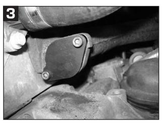
Clean up the face on the exhaust manifold and fit the new blanking plate using the existing pins and some exhaust assembly paste if needed.
