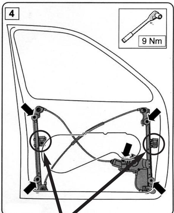
**IMPORTANT NOTE** - Window clamps to be tightened to 6Nm & locked in place with locking nut.
