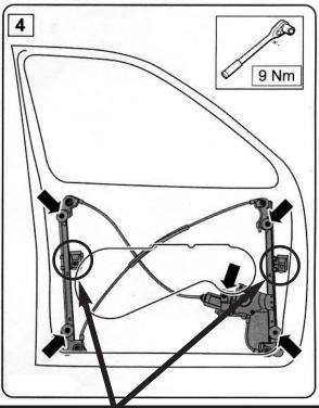
IMPORTANT NOTE - Window clamps to be tightened to 6Nm & locked in place with locking nut.
