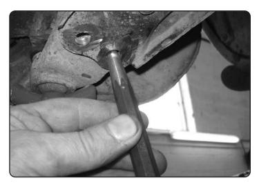
Using a angle grinder grind off the heads of the three rivets underneath the arm, then using a hammer and punch drive out the rivets.
