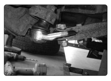
Fit new ball joint with the three M10 nuts and bolts provided and tighten the bolts to 40lbs ft.
