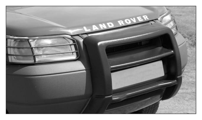
Using the 8mm bolts provided attach the brackets to the A bar. Small brackets to the top, short angle to the bolt end.
