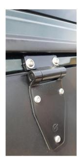
6. Carefully Fit 14mm long St/Stl Riv Bushes into drilled holes.(Riv Bush tool required)
