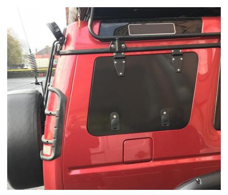
12. Finally, you can lock with supplied keys – and there are grease nipples on the hinges for maintenance.
