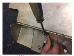
IMPORTANT NOTE: Check the lock mechanism still operates correctly before continuing any further with fitting, otherwise once fitted in the vehicle, it will be virtually impossible to open the lock. Adjust the tab accordingly if the lock cam cannot operate to release the lock pawl.
