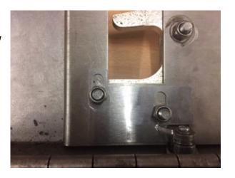
Ensure that the lock claw & pawl are free to move. The nuts want to be tight enough not to rattle, but loose enough to allow free movement.
