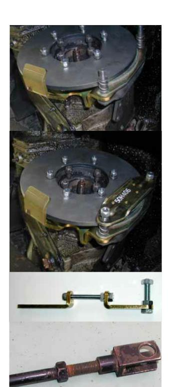
Pass the M10 bolt on the end of the new adjuster through the hole in the handbrake lever vacated by the old push-rod. This is often a bit tight and needs a bit of wiggling.
