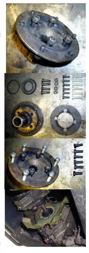
The bottom bolt in the photo has the lock-washer in place and you can see the nut cannot screw fully on to the stud.
