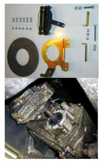
When you remove the drive flange, some oil will leak out of the transfer box - this is normal. If none leaks out - it's empty!
