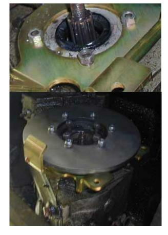
Disassemble the brake calliper as shown. It will need to be assembled in-situ on the back plate.
