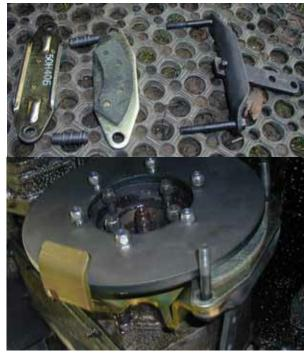
Next slide the spacer tubes and springs over the two bolts, through the holes in the pad and back plate.
