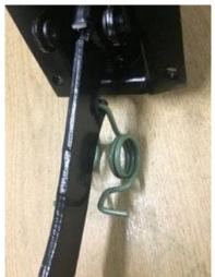
Once the bushes are installed, start by clipping the spring into the pedal bush.
