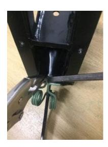
Once the spring has started into the bush, use a flat headed screwdriver to apply pressure while removing the mole grips- then push the spring further into the bush.
