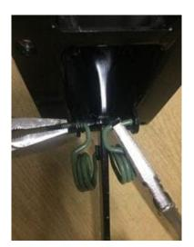
Now grip the other side of the spring and push it into the bush hole - on this side we prefer to pull the spring from the bottom of the footwell into place.
