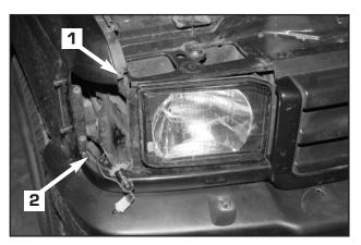
3. The panel below the headlight needs to be removed both sides. There is a screw here (2 on photo above) which is accessible from through the wheel arch with a screwdriver, remove this then lift the end up slightly and pull out to the side of the vehicle.
