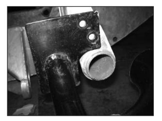
Pre-2001 vehicles will require holes to be drilled in the chassis outriggers.
