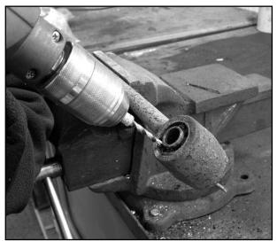
**Step 1**Drill around the bush inner sleeve to remove as much rubber as possible. Turn over and repeat the process.
